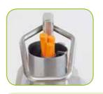
Cylindrical hopper (Ø 58 mm) ensuring a uniform cut for long items.
